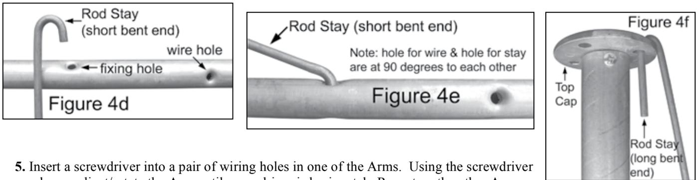
5. Insert a screwdriver into a pair of wiring holes in one of the Arms. Using the screwdriver as a lever, adjust/rotate the Arm until screwdriver is horizontal. Repeat on the other Arms.
