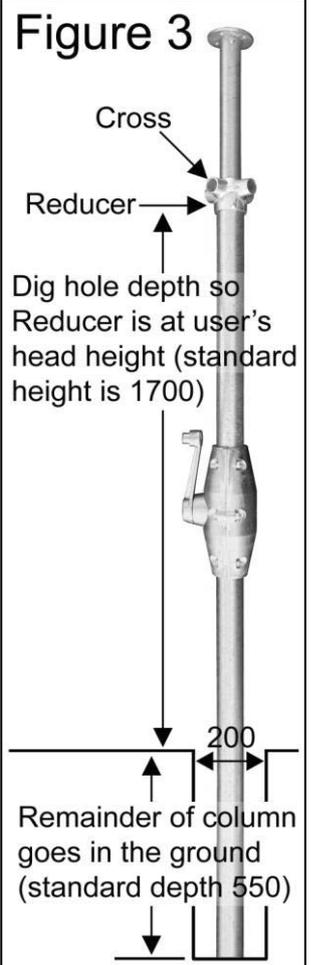
**3a. Hoists with Plastic Handle Casing (Elite, Deluxe & Special):** Remove the column from the hole and insert the Steel Rod through the pre-drilled holes in the bottom of the column. Place column back in the hole. Other models do not require Steel Rod, they have pressed ends to hold firm in the concrete.
